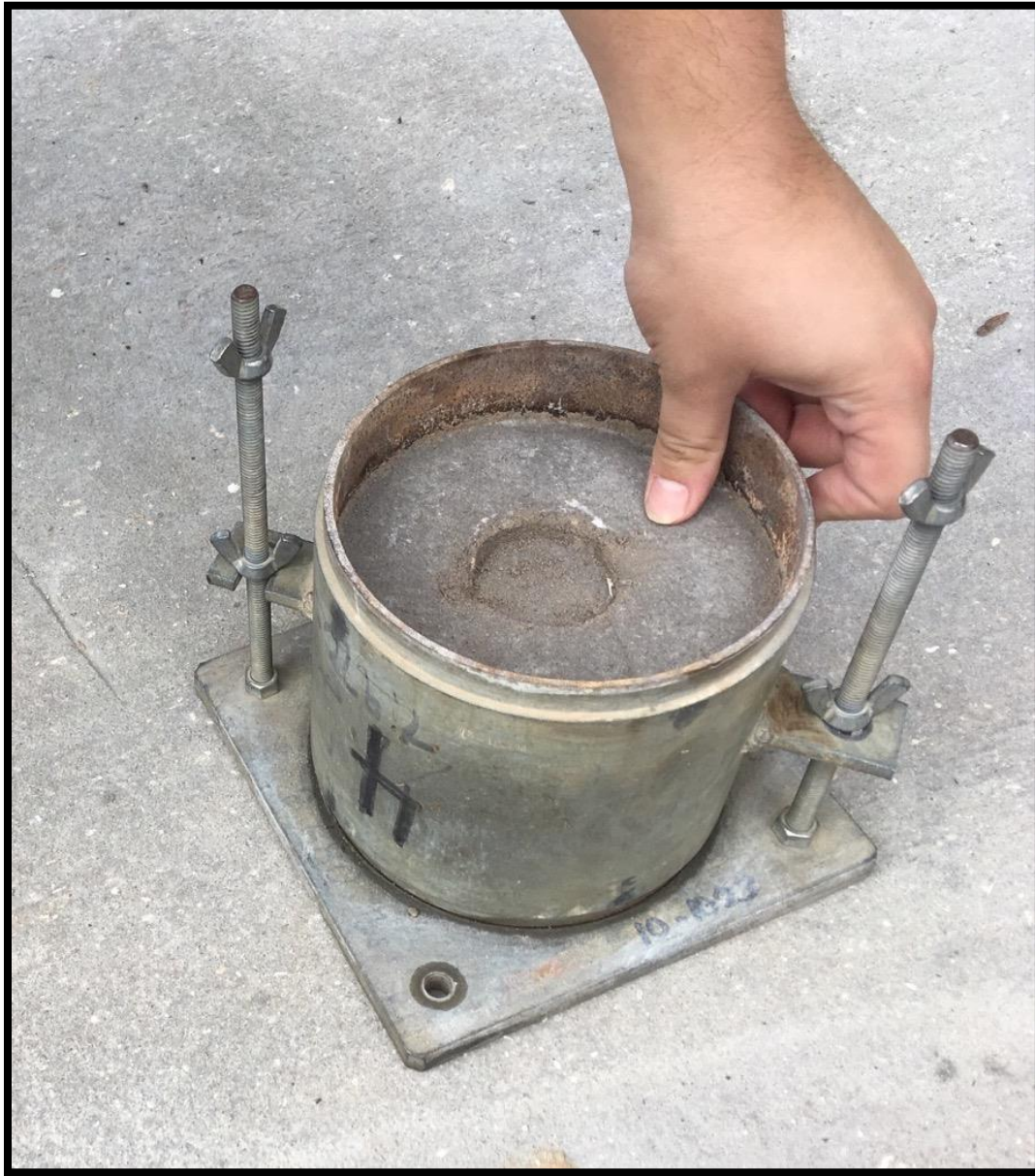
1 Photo of Sample with 2% CONSOLID after LBR Penetration
