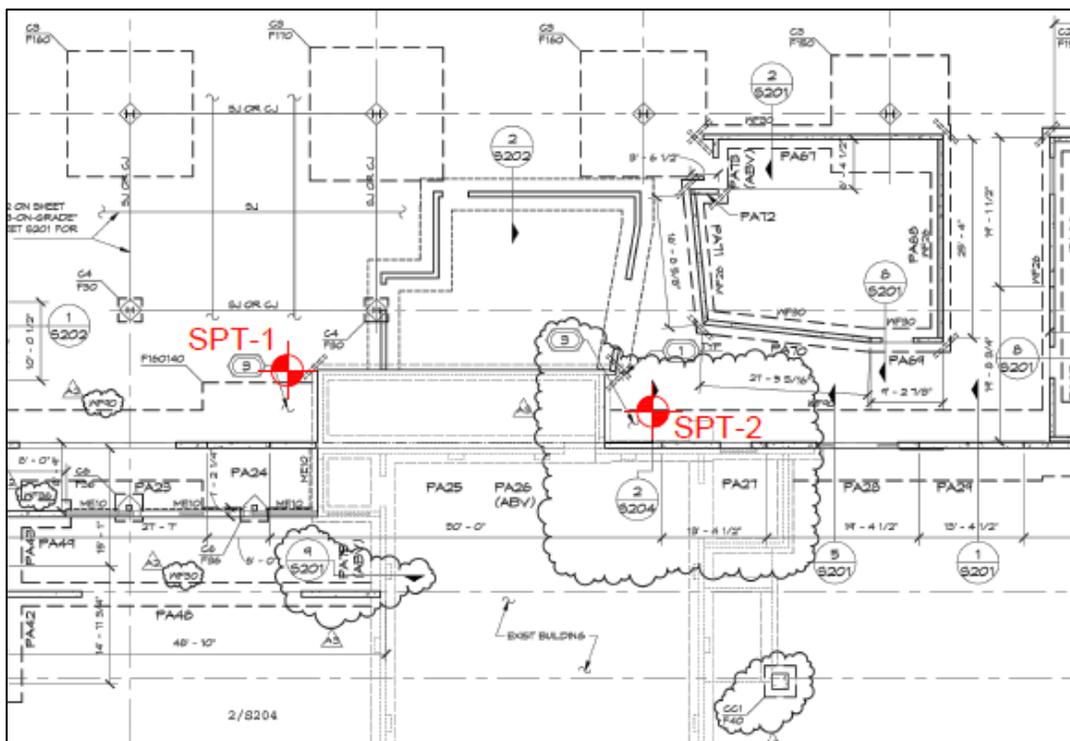
Photo 2, SPT boring locations relative to the existing and proposed buildings
